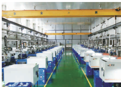
CNC Horizontal Injection Molding Machine
